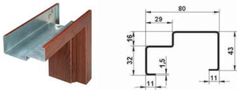
ASYMMETRICAL DOOR FRAME WITHOUT SEALING FB (for TT i GTT door)
