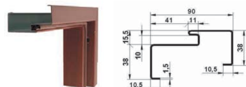
ASYMMETRICAL DOOR FRAME WITH SEALING FA (for TT PLUS, TT MAX, GTT PLUS, GTT MAX door)
