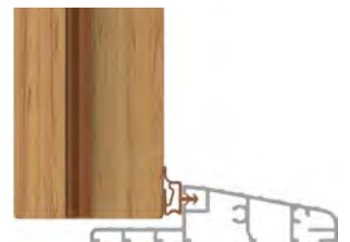
threshold with sealing
